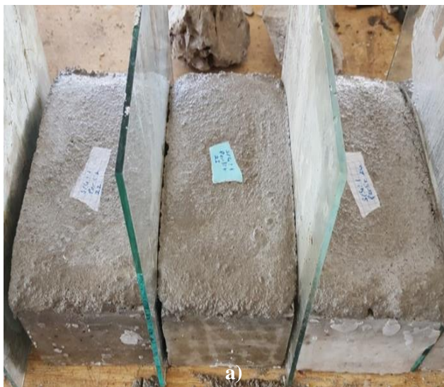
Figure (3): Freezing-thawing treatment: a) Specimens in moulds; b) Specimens in F/T chamber
