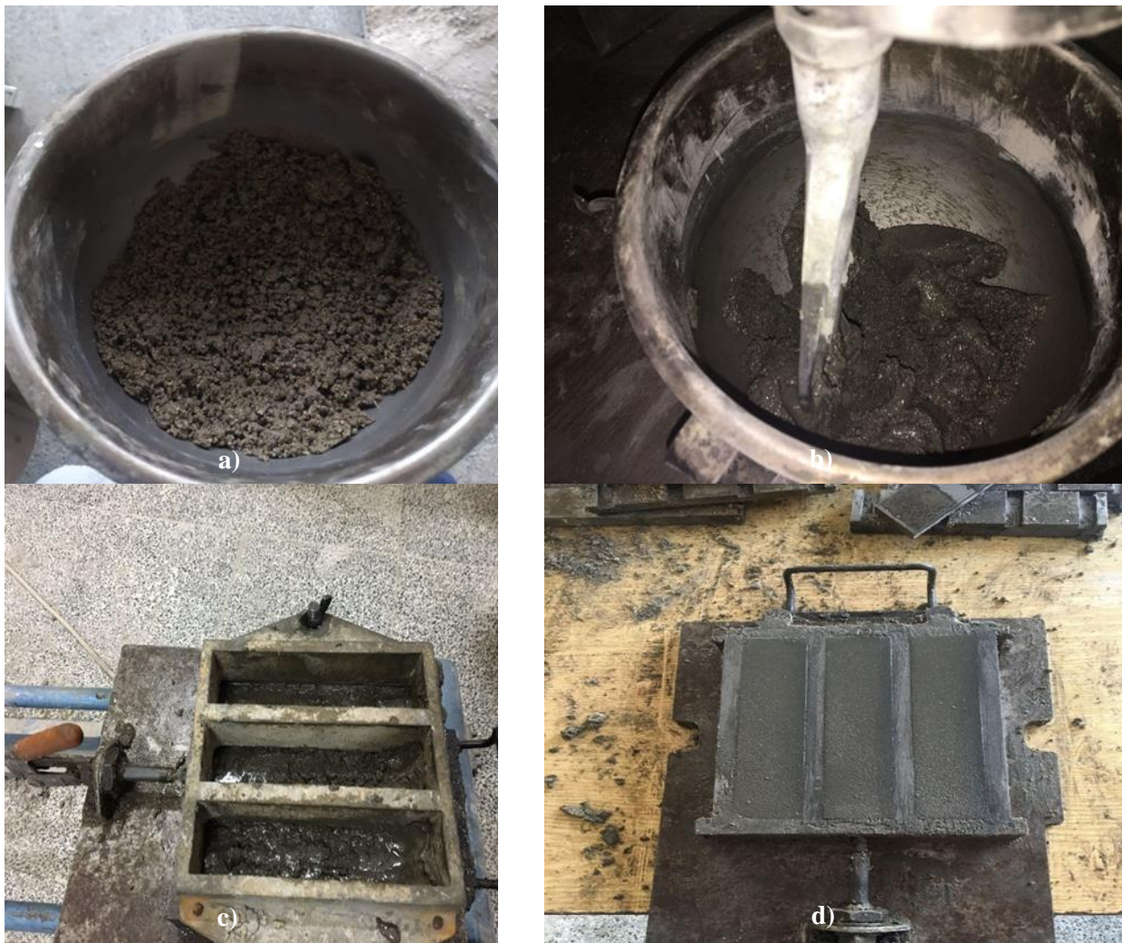
Figure (1): Step-by-step representation of the specimen preparation process: a) Materials used for mortar preparation; b) Mixing phase; c) Mould prepared for casting; d) Specimens' casting in moulds
