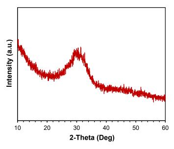
Figure 3. XRD profile of the slag sample.
