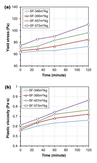
Figure 6. Effect of the fineness of slag on yield stress (a) and plastic viscosity (b) of CPB.
