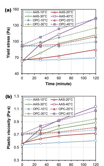
Figure 7. Time-dependent evolution of yield stress (a) and plastic viscosity (b) of CPB.
