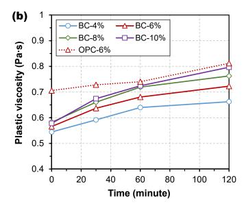
Figure 4. Yield stress (a) and plastic viscosity (b) of CPBs with different binder contents.
