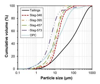
Figure 1. Grain-size distribution curves of tailings and binders.
