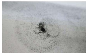
(b) BC-Fe's response to the magnet in circular direction on a A4 paper
