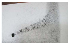
(a) BC-Fe's response to the magnet in line direction on a A4 paper
