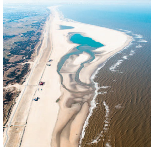
Şekil 2. Hollanda’da 2011 yılında yapılan mega besleme projesi (Mega nourishment project in Netherlands, which was built in 2011)
