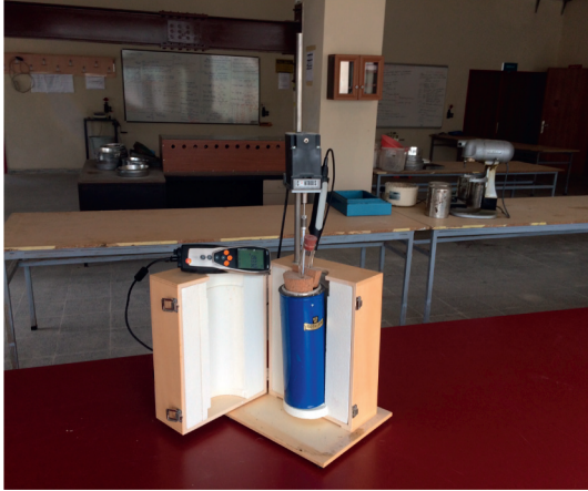
FIGURE 4: Photo of the calorimeter used by the chemical technique.
