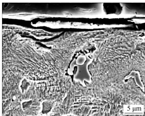
Fig. 16 Subsurface microstructure of wear sample of SAE 65 bronze
