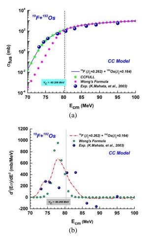
**Fig. 3.** Graphs of (a) the cross-sections and (b) barrier distributions for  ${}^{19}F + {}^{192}Os$  the fusion reaction within the coupled channel (CC) model the interactions of the deformed (rotational) projectile and target nuclei.
