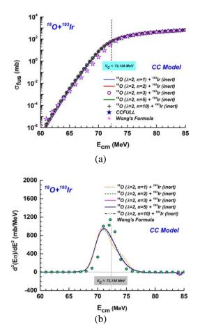
**Fig. 4.** Graphs of (a) the cross-sections and (b) barrier distributions for  ${}^{18}O + {}^{193}Ir$  the fusion reaction within the coupled channel (CC) model the interactions quadrupole (2<sup>+</sup>) state of projectile nuclei and inert target nuclei.
