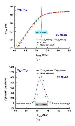
**Fig. 6.** Graphs of (a) the cross-sections and (b) barrier distributions for  ${}^{18}O + {}^{193}Ir$  the fusion reaction within the coupled channel (CC) model the interactions of the deformed (rotational) projectile and target nuclei.
