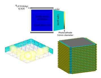
Figure 12: CHANDLER-like detector concepts [25, 26, 27, 28]. 3D segmentation and 2D light collection that is based on Raghavan Optical Lattice [15]. Light is transported along rows and columns of cells by total internal reflection.
