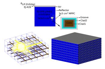
Figure 13: SOLID-like detector concepts [29, 30, 31, 32, 33, 34]. 3D segmentation and 2D light collection.
