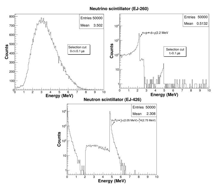
Figure 15: Total deposited energy distribution in neutrino scintillators (top) and neutron scintillators (bottom). For the top plots, two different time cuts are applied as calculating total deposited energy in neutrino scintillators.
