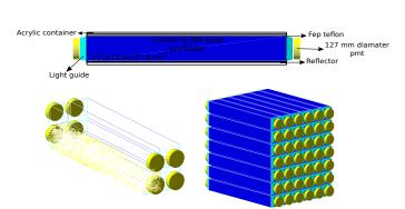
Figure 8: PROSPECT-like detector concepts [16, 17, 18, 19]. 2D segmentation and 1D light collection.
