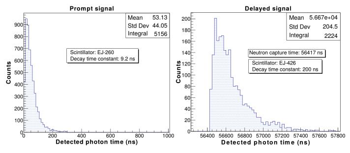
Figure 14: Prompt and delayed components of an anti-neutrino signal obtained with Chandler-style detector. Pulse shape discrimination is an effective method for discriminating prompt and delayed signals in this type of detector.
