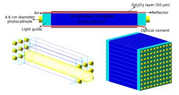
Figure 10: PANDA-like detector concepts [21, 22]. 2D segmentation and 1D light collection.
