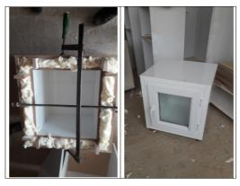
Figure 3. The production of the cooled cabinet
