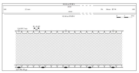
Figure 3. Technical plan of monofilament gillnet with 22 mm mesh size
