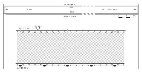
Figure 2. Technical plan of monofilament gillnet with 20 mm mesh size
