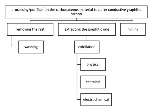
Figure 4. Processing the carbonaceous mixture
