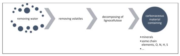
Figure 3. The general pathway to fixed carbon from biomass by heat treatment
