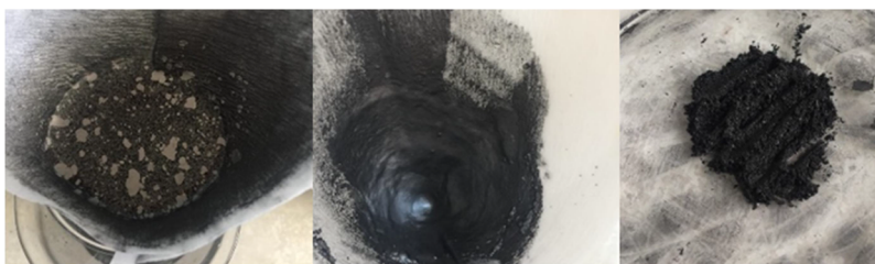
Figure 1. Graphene was obtained from graphite at room temperature.
