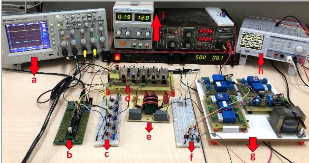
Fig. 16. The experimental setup (a: oscilloscope, b: TMS320DOCKF28335 kit c: isolation circuit d: H5 inverter and drive, e: Filter, f: Analog circuit, g: voltage sensor circuits, h: voltage analyzer, i: DC Supplies.)
