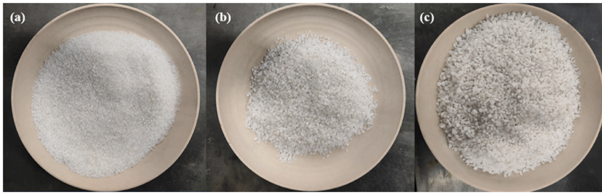
Fig. 1. Particle diameter gradations of gravel rocks: (a) 1–2 mm; (b) 2–4 mm; (c) 4–6 mm.
