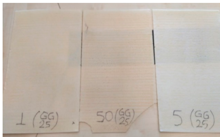
Figure 7. Wafer sheets produced on GG-25 cast-iron baking plates at a production rate of 31 pcs/min.
