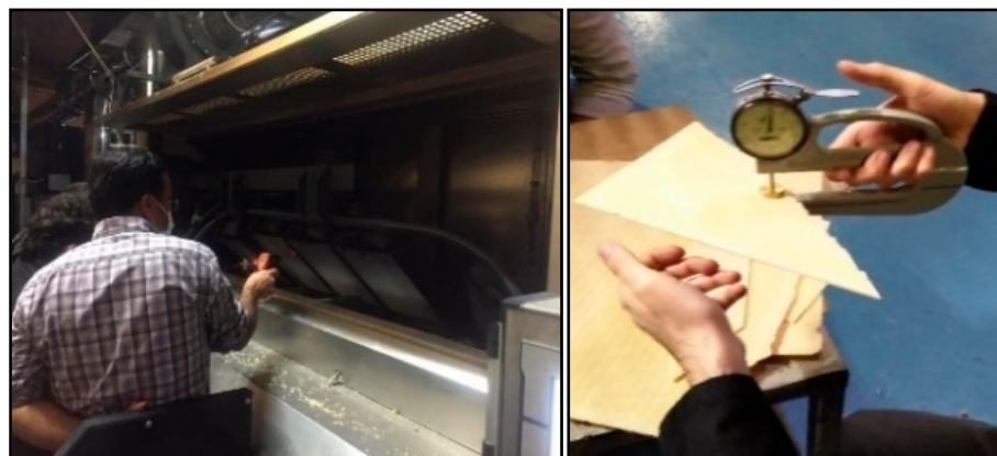
Figure 5. Temperature measurement of baking plates during period of wafer production and thickness measurement of the wafer sheet.
