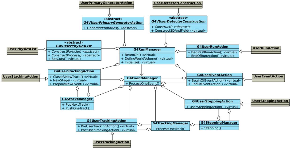
Figure 1: Unified Modeling Language (UML) class diagram of a typical Geant4 application. The blue color shows classes provided by Geant4, and the brown color indicates concrete classes to be written by the application developers.
