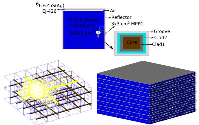
Figure 13: SOLID-like detector concepts [29, 30, 31, 32, 33, 34]. 3D segmentation and 2D light collection.
