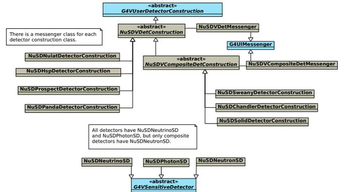
Figure 2: The UML diagram of the classes involved in building NuSD detectors.
