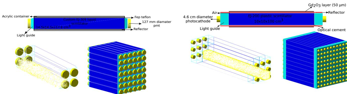
Figure 8: PROSPECT-like detector concepts [16, 17, 18, 19]. 2D segmentation and 1D light collection.
