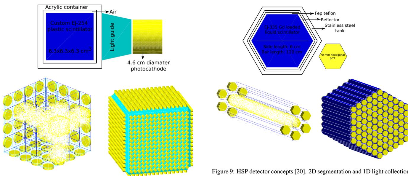
Figure 9: HSP detector concepts [20]. 2D segmentation and 1D light collection.
