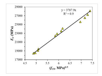
**Fig. 5.** Relationship between  $f_{CS}$  and  $E_C$  of concrete irrespective of strength class and HSF volume.
