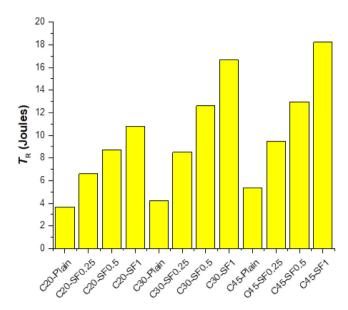
**Fig. 9.** Flexural toughness  $(T_R)$  of C20, C30 and C45 concrete classes with the varying HSF volume.
