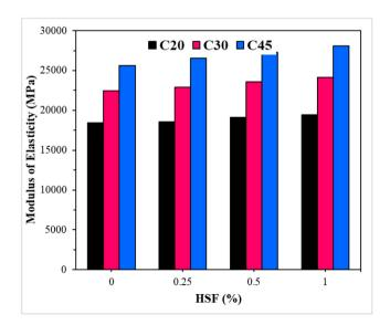
**Fig. 4.**  $E_C$  of each strength class with the varying HSF volume.
