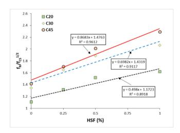
**Fig. 7.** Relationship between  $f_R/f_{CS}^{0.5}$  of each strength class and HSF (%).
