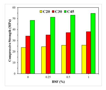
Fig. 3. Compressive testing results of each strength class with the HSF volume.
