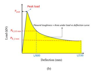
Fig. 2. Overview of (a) flexural testing setup (b) typical load versus mid-span deflection curve.
