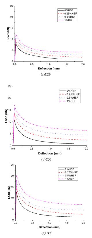
**Fig. 8.** Load-deflection behavior of (a) C20 strength class (b) C30 strength class and (c) C45 strength class with the variation in HSF volume.
