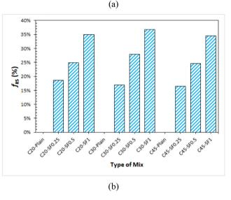
**Fig. 10.** (a)  $f_{RS}$  of C20, C30 and C45 classes of concrete with the varying HSF volume at the deflections of L/600 and L/150 i.e. 0.5 mm and 2 mm (b)  $f_{RS}$  as the percentage of peak strength or  $f_{R}$ .
