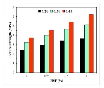
**Fig. 6.**  $f_R$  of each strength class with the varying HSF volume.
