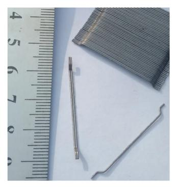
Fig. 1. Hooked steel fiber (HSF).
