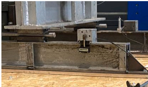
Fig. 22. Position of inclinometers on the loading beams.
