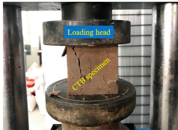
Figure 6. A cubic CTB sample subjected to the unconfined compressive strength (UCS) test.
