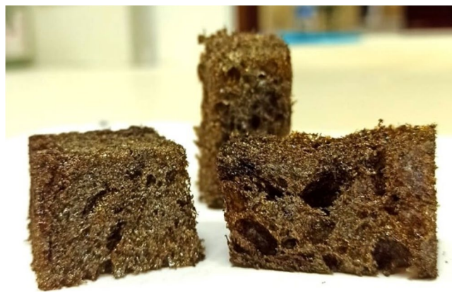
Fig. 1 Carbon foams obtained from sucrose with 10% concentrations of \text{Zn}(\text{NO}_3)_2
