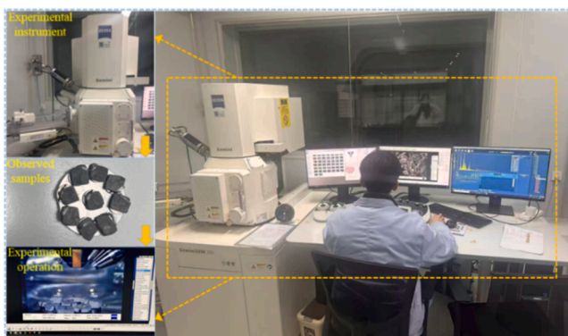
Fig. 7. Creation, curing and testing steps for SEM-EDS specimens.
