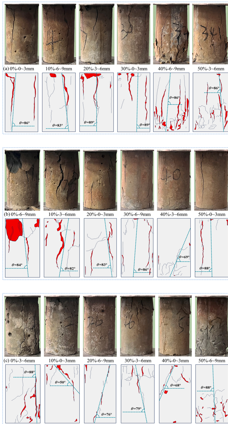
Fig. 13. Failure modes of 56-day cured specimens having a c/t ratio of (a) 1:4; (b) 1:6; and (c) 1:8.
