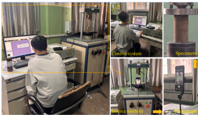
Fig. 6. Photos regarding UCS test's application and evaluation.
